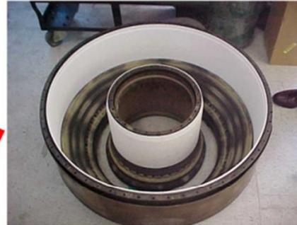
Solar Turbines combustor liner. 25,000+ hrs (completed 2006)
