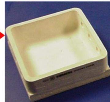
Blade Tip Seals engine tested
