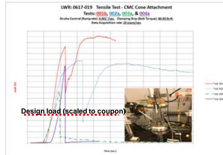
**3X Static design load capability – Fatigue testing in progress**
